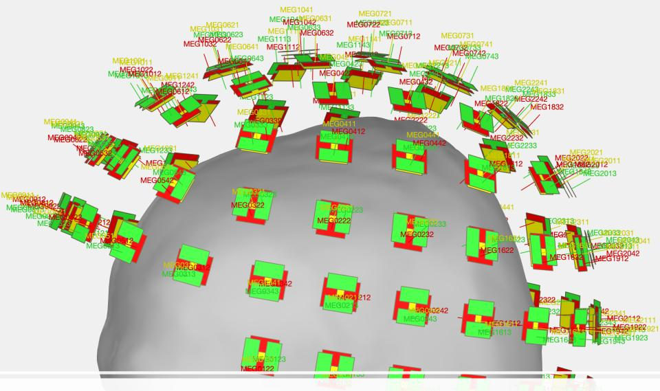
The Mixed Sensor Array – MAGS and GRADS
